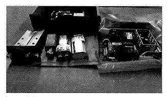
(2)Motorola TENSR power supply, (2)Gentea Capacitors, Condor Power supply, unknown power supply module, LIP power sensor
