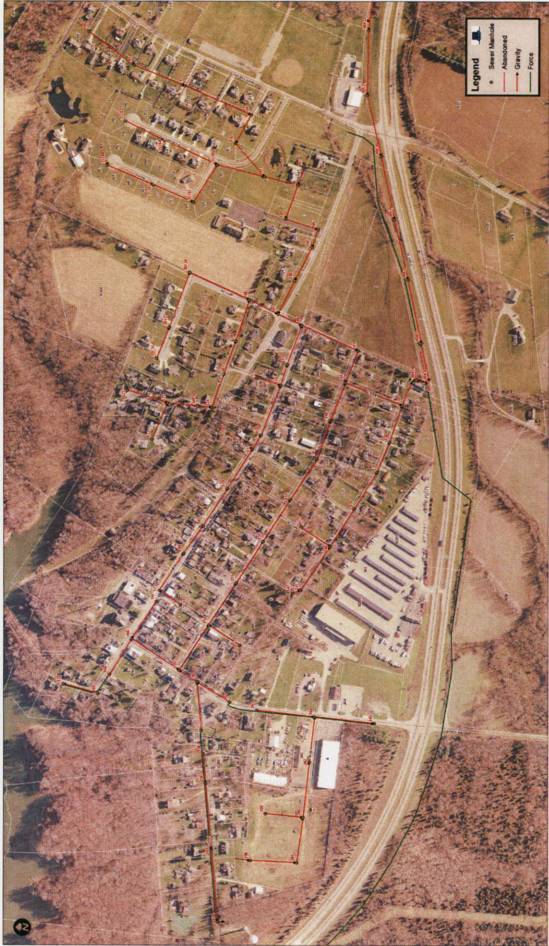
Village of Harveysburg - Sanitary Sewer System
